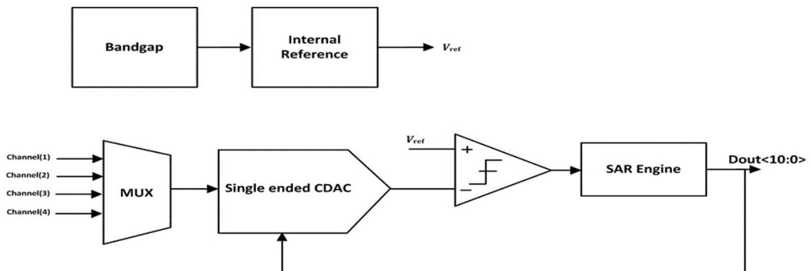
The ADC reference voltage can be either generated internally or set externally via one of the two available mixed-signal GPIO pins on the ATBTLC1000.
