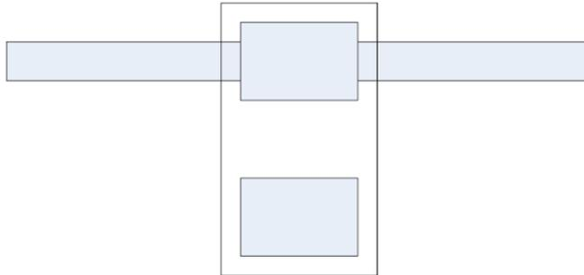
The following figure shows a stub route to the capacitor pad. This should be avoided, as it adds additional impedance in series with the capacitor.
