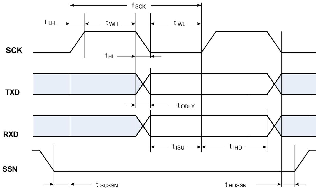
**Table 11-10. ATBTLC1000 SPI Slave Timing Parameters <sup>(1)</sup>**
