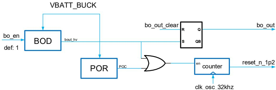
**Figure 6-5. ATBTLC1000 POR and BOD Timing Sequence**
