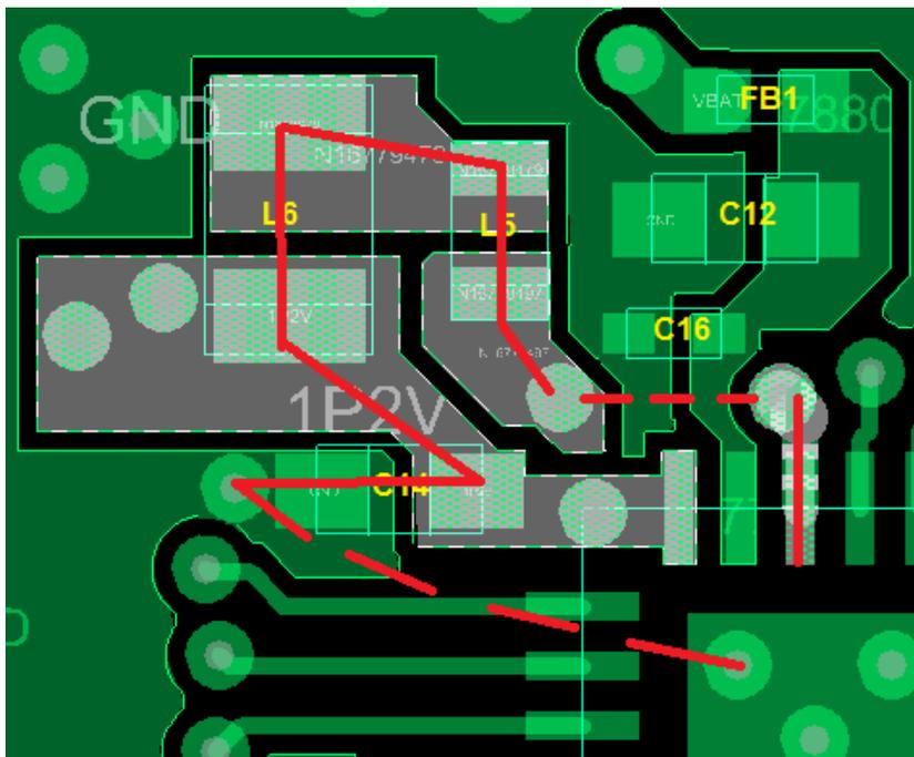
The current loop described above is indicated by the red line, with the dashed portions indicating the path on inner layers. The route from pin 14 to L5 is on an inner layer and is shown in the following figure in red/white.
