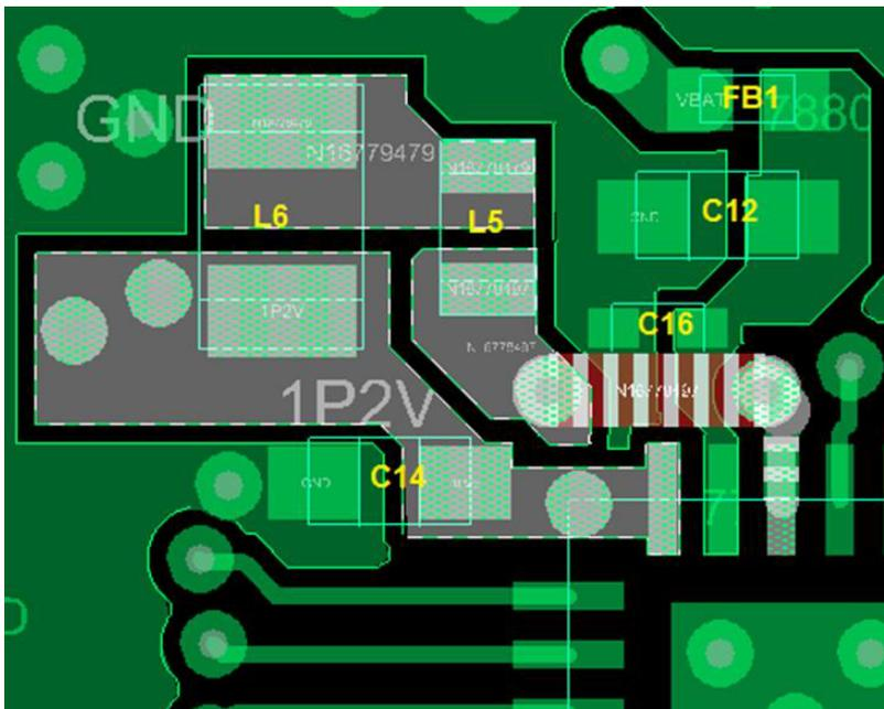
Placement of FB1, C12, and C16 should be as close as possible to the VBAT\_BUCK pin (pin 15), with the smaller capacitor, C16, placed closest to the pin. Again, the route should be as heavy as possible to provide a low-impedance path. The placement and routing of these components is shown in [Figure 15-2](#).
