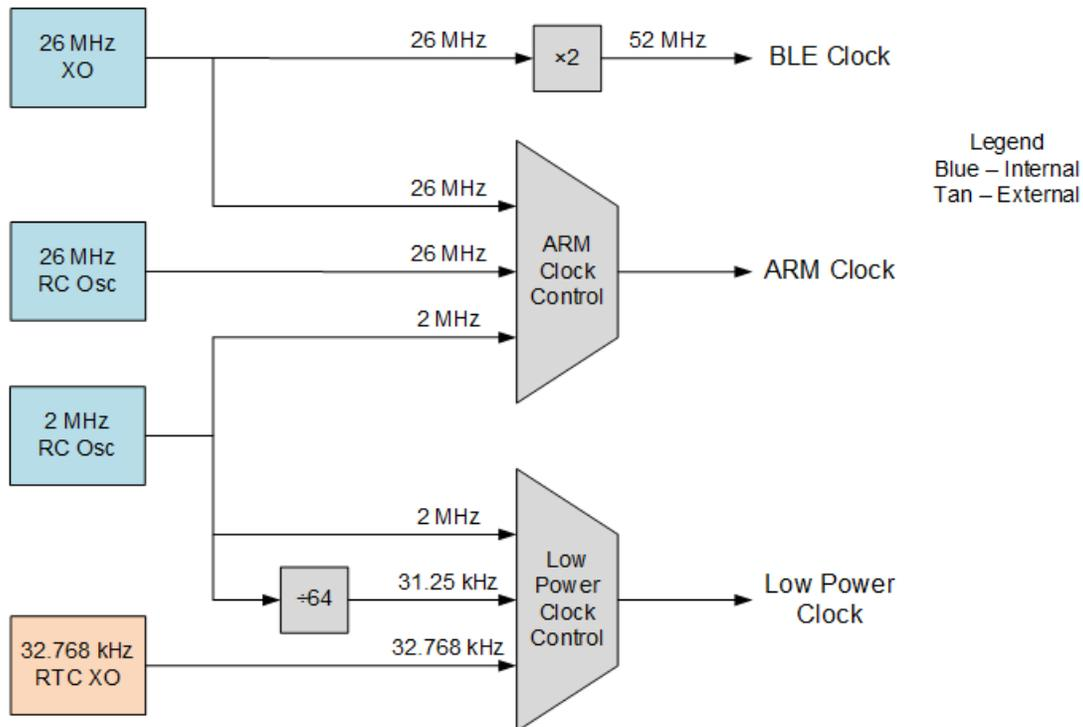
The BLE Clock is used to drive the BLE subsystem. The ARM clock is used to drive the Cortex-M0 MCU and its interfaces (UART, SPI, and I<sup>2</sup>C). The recommended MCU clock speed is 26 MHz. The Low Power Clock is used to drive all the low-power applications like the BLE sleep timer, always-on power sequencer, always-on timer, and others.
