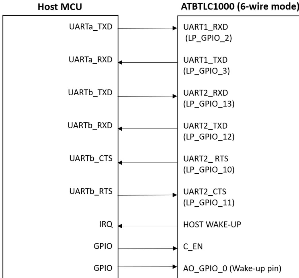
The host wake-up pin from ATBTLC1000 can be connected to any interrupt pin of the host MCU. The host MCU can monitor this pin level and decide to wake up based on events from ATBTLC1000.
