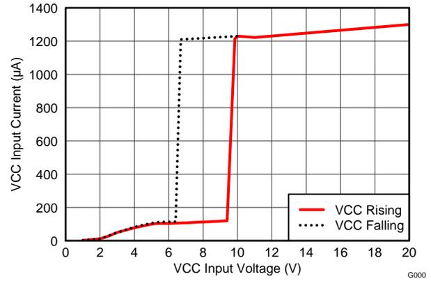
Figure 2. VCC Input Current vs Vcc Input Voltage
