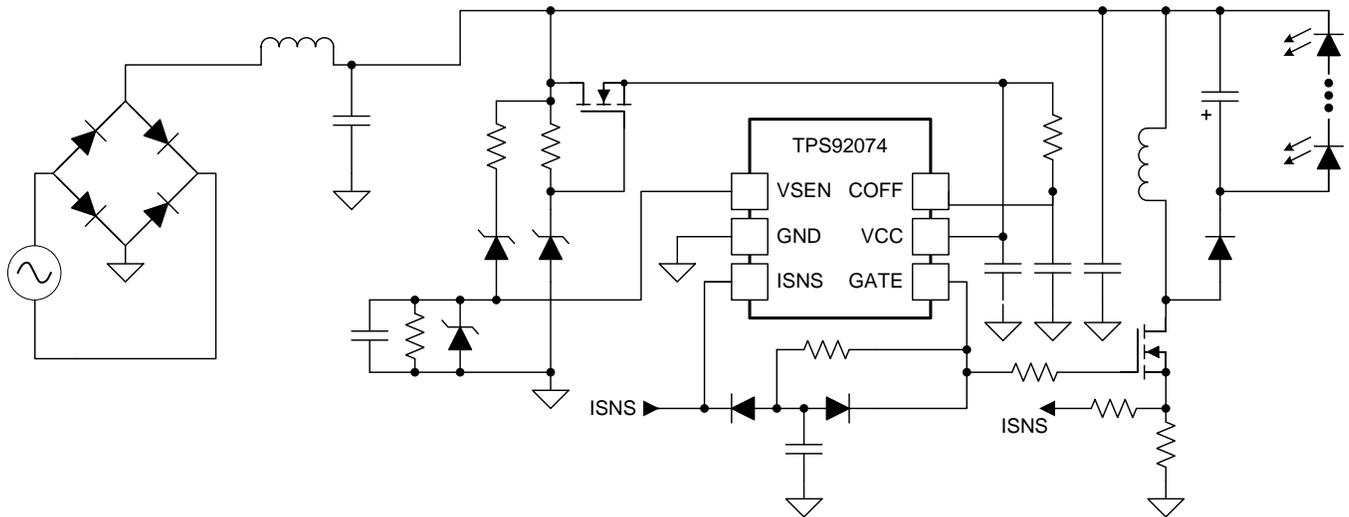
Figure 17. TPS92074 Buck-Boost Topology with DC Side Filter
