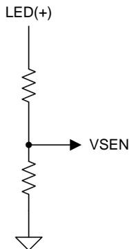
**Figure 13. Voltage Sense for Low Voltage Buck Applications**
