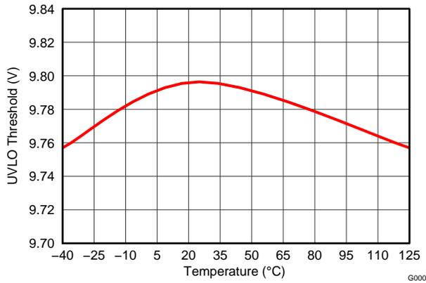
Figure 3. Input Voltage (UVLO Rising) vs Junction Temperature
