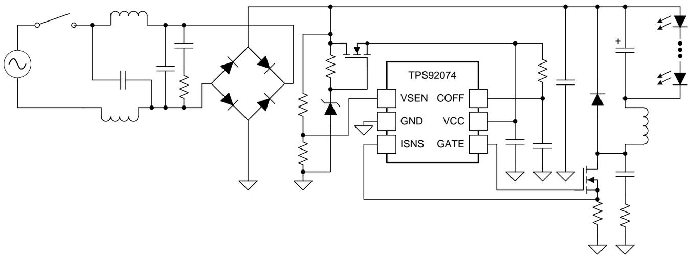
Figure 16. TPS92074 Buck Topology with AC Side Filter
