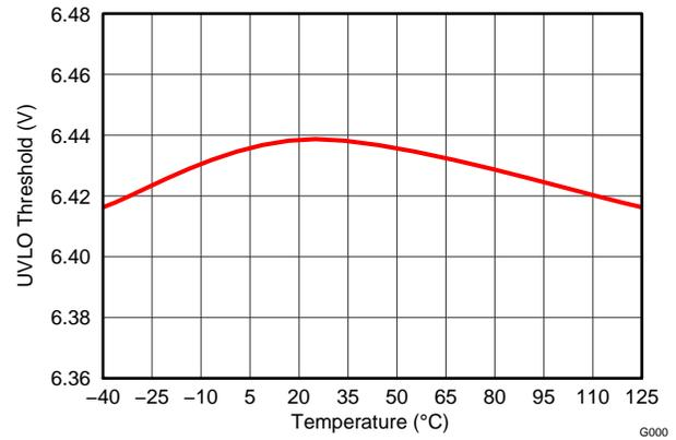
Figure 4. Input Voltage (UVLO Falling) vs Junction Temperature
