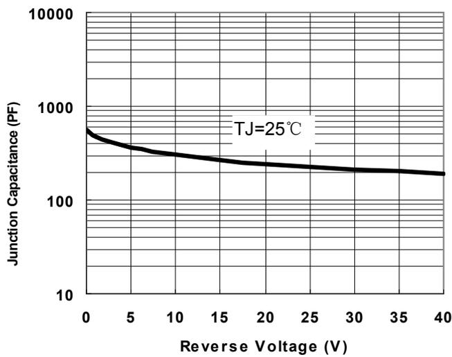
Fig.1-Typical Junction Capacitance
