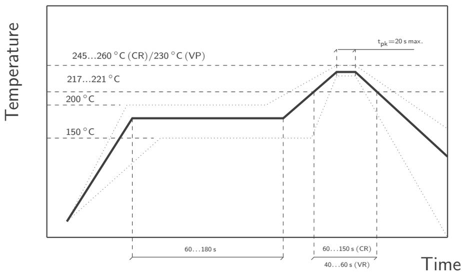
Recommended reflow soldering conditions following IPS/JEDEC J-STD-020.
