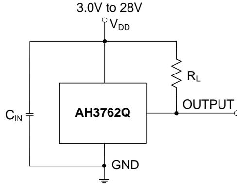
Note: 4.  $C_{IN}$  is for power stabilization and to strengthen the noise immunity, the recommended capacitance is 10nF to 100nF.  $R_L$  is the pull-up resistor.
