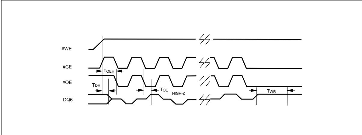
Page Write Timing Diagram Software Data Protection Mode
