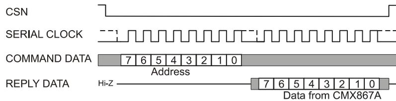
**e) One Address byte from  $\mu\text{C}$  and 2 Reply bytes from CMX867A**
