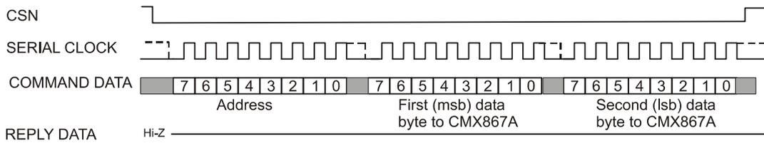
**d) One Address byte from  $\mu\text{C}$  and one Reply byte from CMX867A**
