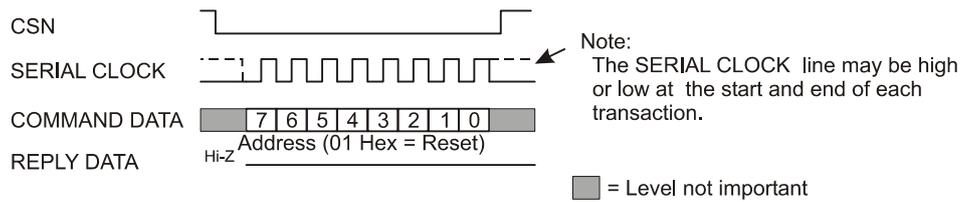
**b) One Address and one Data byte from  $\mu\text{C}$**
