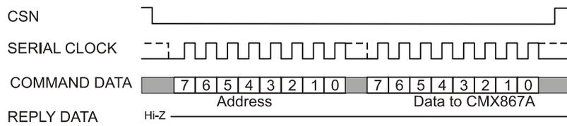
**c) One Address and 2 Data bytes from  $\mu\text{C}$**
