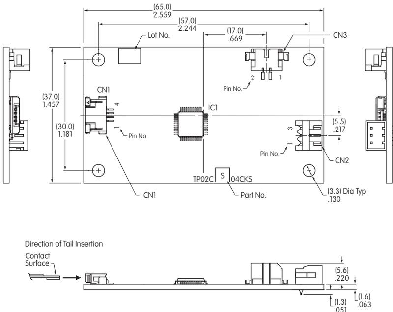
CN1 4-Wire Analog Touch Screen Connector - 4 Pins
