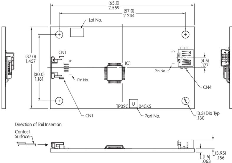
CN1 4-Wire Analog Touch Screen Connector - 4 Pins
