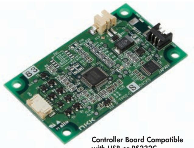
**Controller Board Compatible with USB or RS232C**
