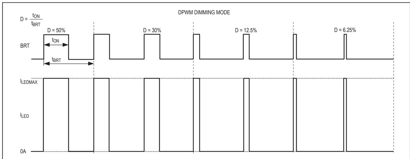
Figure 5. LED Current Control Using DPWM Dimming Mode
